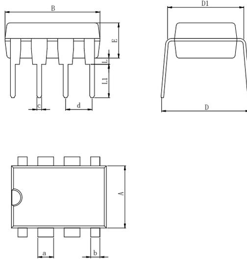
Dimensions In Millimeters(DIP-8)
