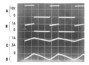
$V_{OUT} = 5V$ A: Output Pin Voltage, 10V/div B: Output Pin Current, 1A/div C: Inductor Current. 0.5A/div D: Output Ripple Voltage, 20 mV/div,
