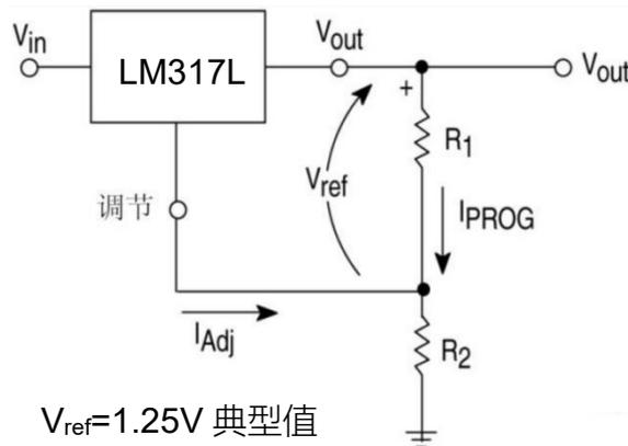
稳压输出电压由下式给出:  $V_{out} = V_{ref} * (1 + R_2/R_1) + I_{adj} * R_2$
