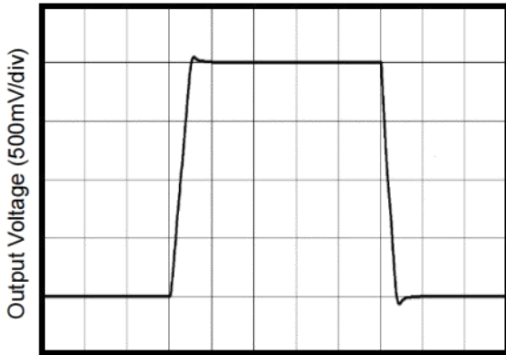
Non-Inverting Large-Signal Step Response
