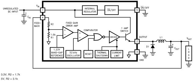
5V, R2 = 3.1k 12V, R2 = 8.84k 15V, R2 = 11.3k For ADJ. Version R1 = Open, R2 =  $0\Omega$ Note: Pin numbers are for the TO-220 package.
