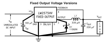
$C_{IN}$  — 100  $\mu$ F, 75V, Aluminum Electrolytic  $C_{OUT}$  — 330  $\mu$ F, 25V, Aluminum Electrolytic D1 — Schottky, 11DQ06 L1 — 330  $\mu$ H, PE-52627 (for 5V in, 3.3V out, use 100  $\mu$ H, PE-92108)
