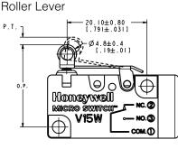
Lever Type "06" Long Roller Lever Ρ.Τ. 29.80±1.50 [1.173±.059] Ø4.8±0.4 [.|9±.0|] (+)Ш Q, Æ G ο.΄ C Honeyvvell NC. (2) MICRO ŠWITCH V15W NO.3 Ф COM.()
