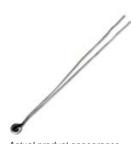
192 Series, Uni-Curve with bare leads and epoxy, 1,000 Ohm resistance, ±1,0 °C [1.8 °F] tolerance, 25/85 BETA = 3348
