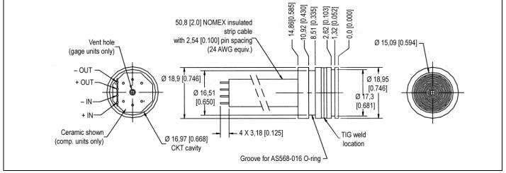
**Note:** Non-concentricity effects at the diaphragm weld area may cause runout of up to  $\pm 0.006$  in between the upper and lower portions of the sensor body. (It is recommended to use a counter bore to mate with this device to allow for this non-concentricity).
