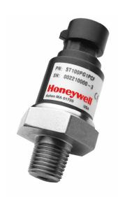
The Model ST pressure transducer combines Honeywell's proven silicon pressure sensing with the latest in ASIC technology in a rugged, industrial package. High value, coupled with outstanding performance, make this an ideal transducer for industrial control applications such as air compressors and pneumatic equipment. Temperature compensated, calibrated, and amplified, the ST has pressure ranges from 0 psi to 5.0 psi to 0 psi to 250 psi.
