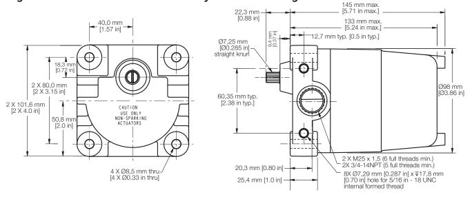
Figure 2. MICRO SWITCH CX - side rotary short housing
