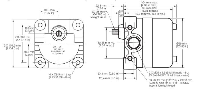
Figure 3. MICRO SWITCH CX - plunger standard and short housing
