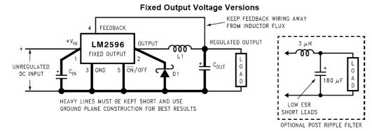
$C_{IN} = 470 \mu F$ , 50V,  $C_{OUT} = 220 \mu F$ , 25V (Aluminum Electrolytic Nichicon "PL Series" D1 = 5A, 40V Schottky Rectifier, IN5825
