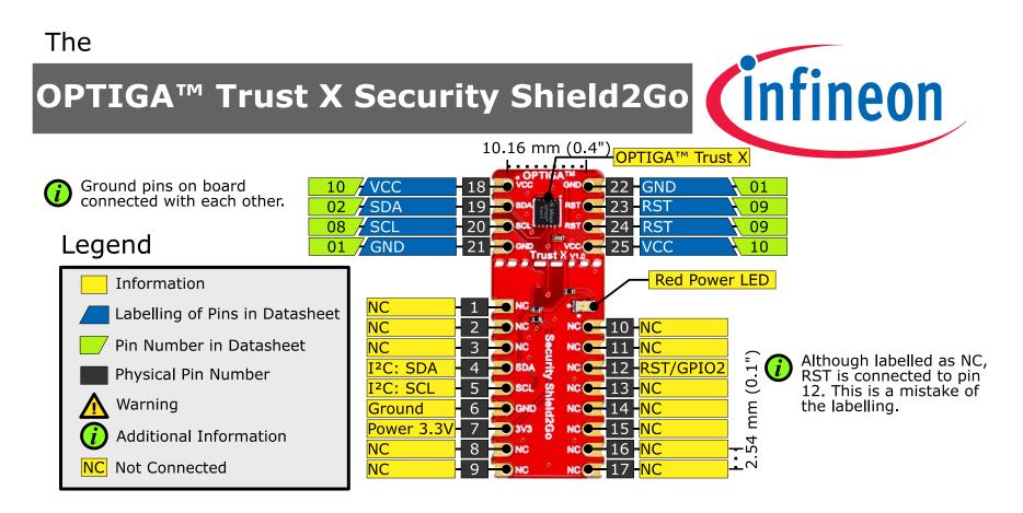
The maximum voltage on VCC pin is 7 V, any other pin VCC+0.3 V.
