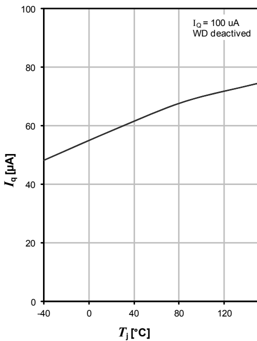
Current Consumption I_q versus Junction Temperature T_j
