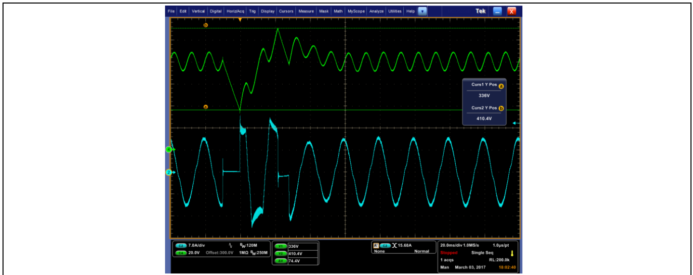
Figure 23 AC line drop out for 10 ms when V_{IN} = 115 V AC at P_{OUT} = 800 W
