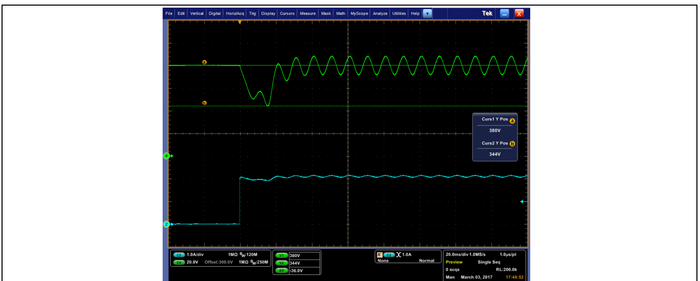
Figure 19 Load step: 0% → 100% at V_{IN} = 230 V AC
