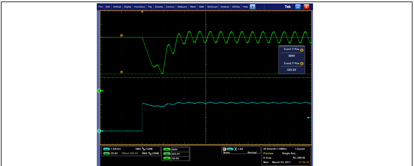
Figure 18 Load step: 0% → 100% at V_{IN} = 115 V AC
