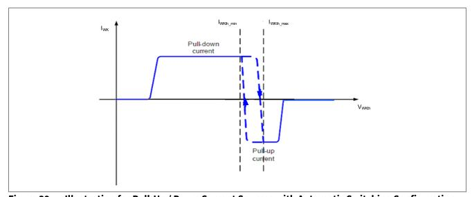
Figure 39 Illustration for Pull-Up / Down Current Sources with Automatic Switching Configuration
