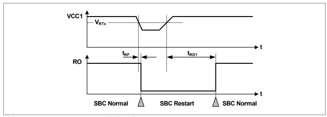
Figure 51 VCC1 Undervoltage Timing Diagram
