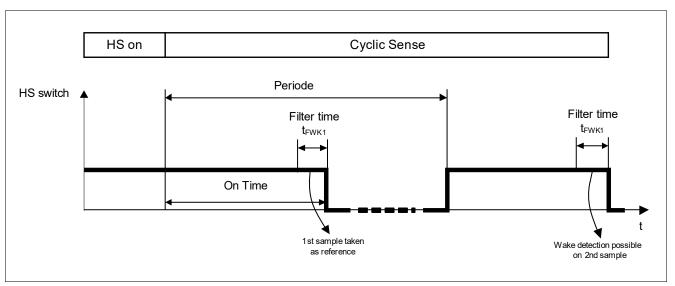
Figure 7 Wake Input Timing
