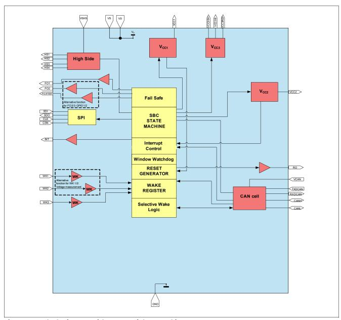
Figure 1 Block Diagram with CAN Partial Networking
