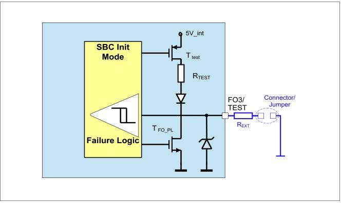
Hint for Increasing the Robustness of pin FO3/TEST during Debugging or Programming Figure 60
