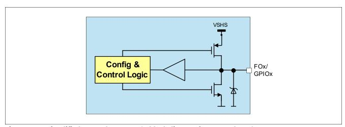
Figure 44 Simplified General Purpose I/O block diagram for FO2 and FO3/TEST
