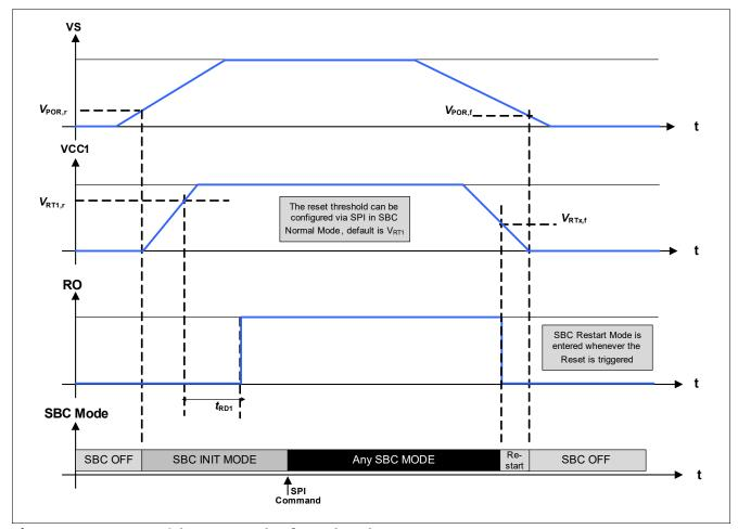
Figure 50 Ramp up / down example of Supply Voltage
