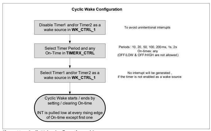
Figure 10 Cyclic Wake: Configuration and Sequence
