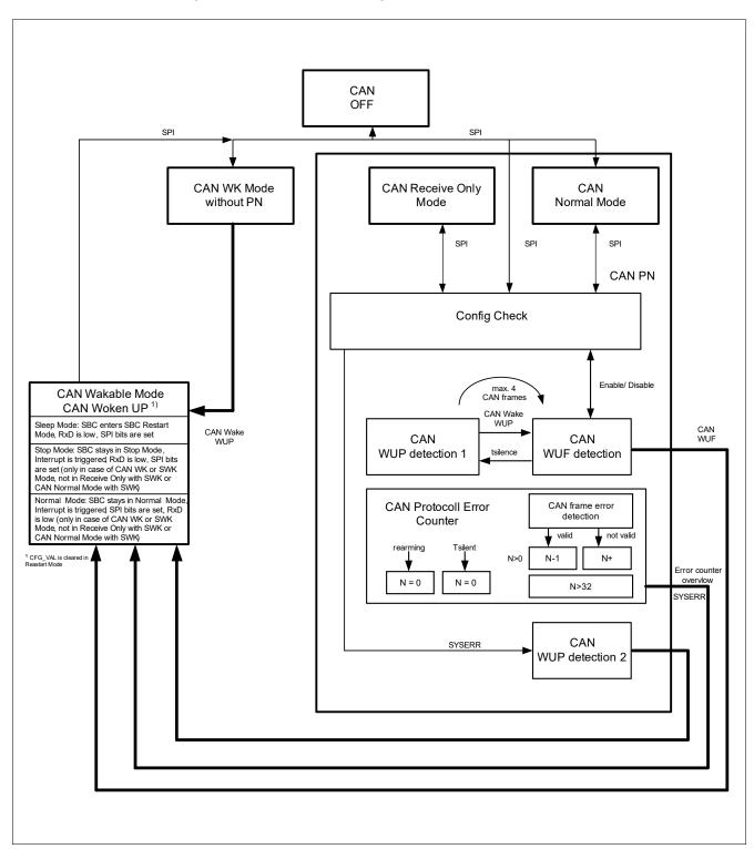
Figure 11 CAN Selective Wake State Diagram
