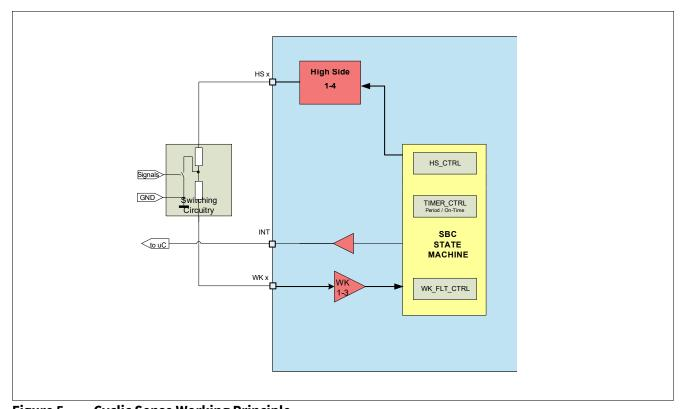
Figure 5 Cyclic Sense Working Principle
