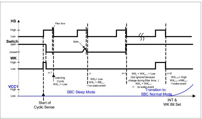
Figure 9 Cyclic Sense Example in SBC Sleep Mode, HSx starts "OFF"/HIGH, GND based WKx input
