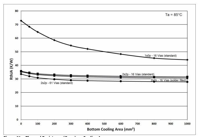
Figure 61 Thermal Resistance ( $R_{th_JA}$ ) vs. Cooling Area
