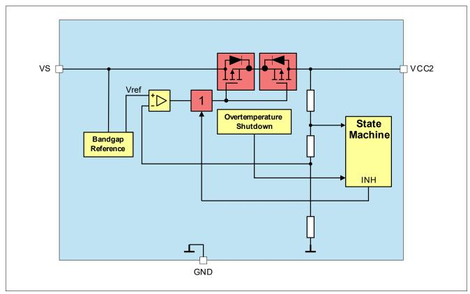
Figure 19 Module Block Diagram
