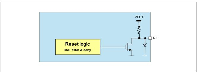
Figure 45 **Reset Block Diagram**
