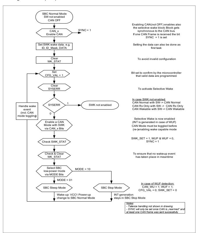
Figure 12 Flow for activation of SWK
