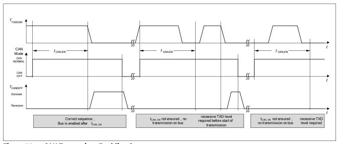
Figure 33 CAN Transceiver Enabling Sequence
