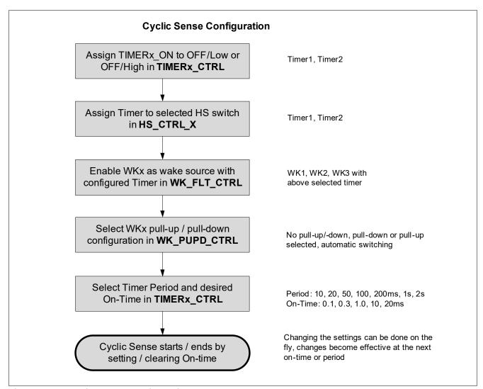
Figure 6 Cyclic Sense: Configuration and Sequence
