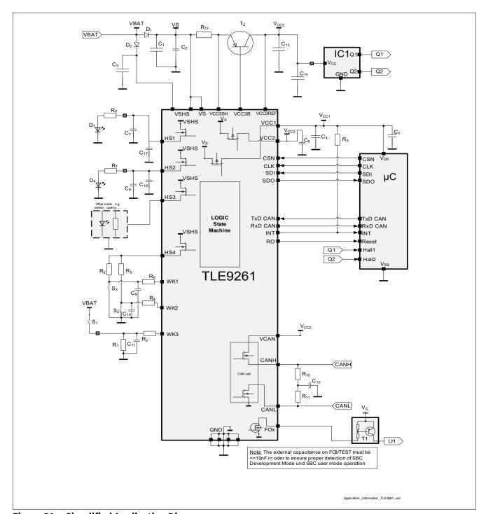
Figure 58 Simplified Application Diagram
