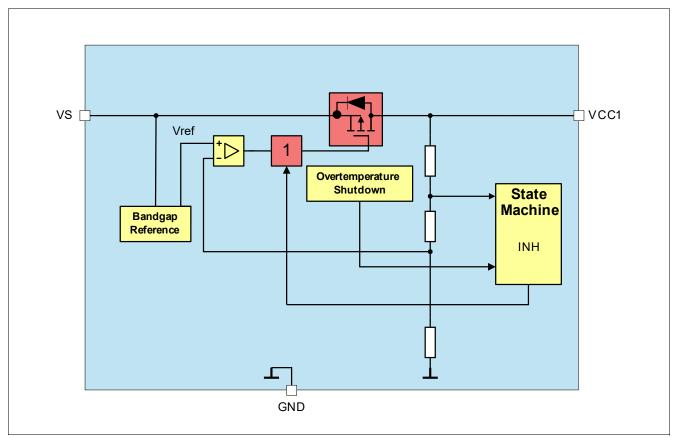
Figure 16 **Module Block Diagram**
