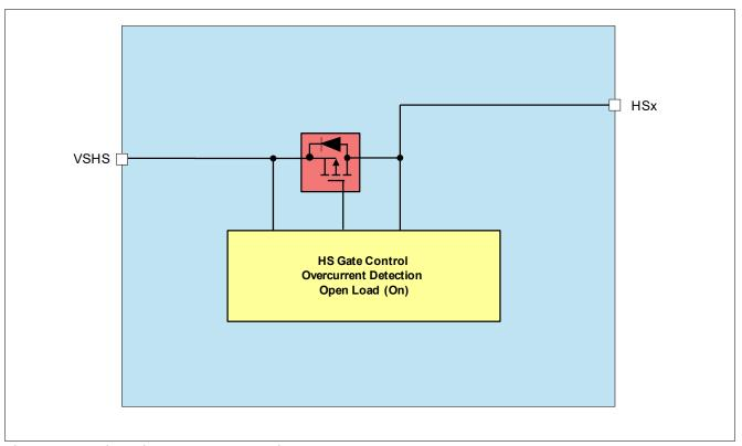
Figure 29 High-Side Module Block Diagram
