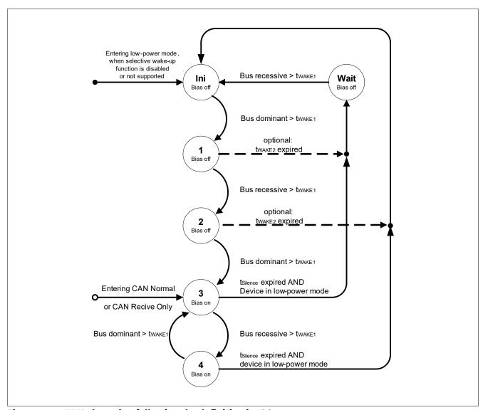
Figure 34 WUP detection following the definition in ISO 11898-2:2016
