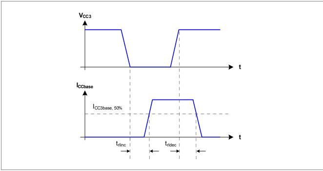
Figure 26 Regulator Reaction Time
