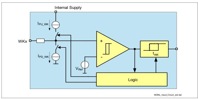
Figure 37 **Wake Input Block Diagram**
