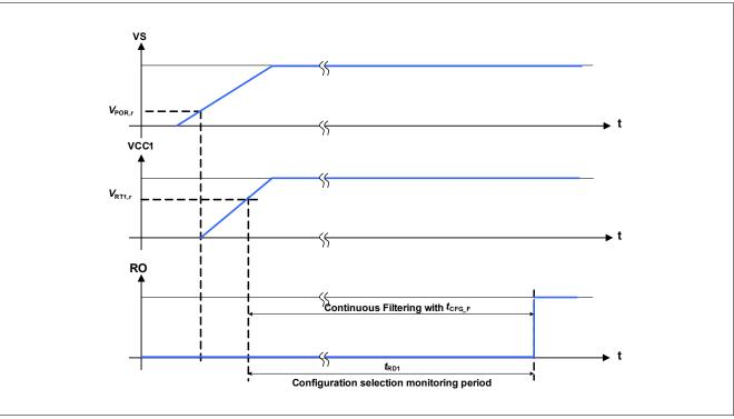
Figure 4 Hardware Configuration Selection Timing Diagram
