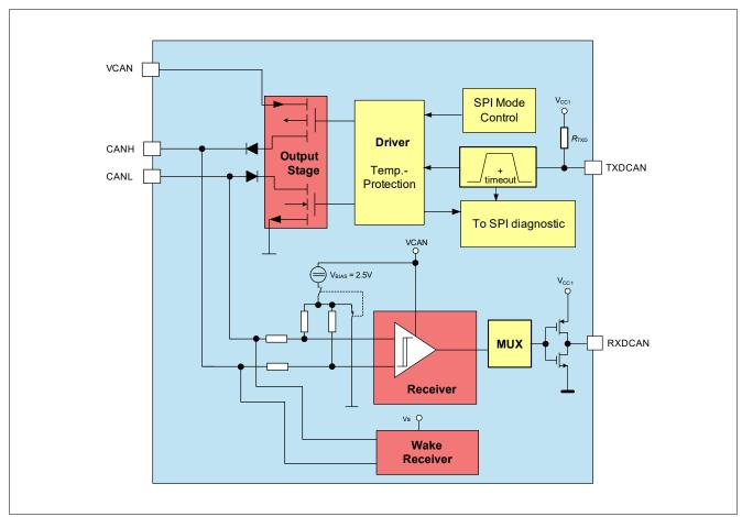
Figure 30 Functional Block Diagram
