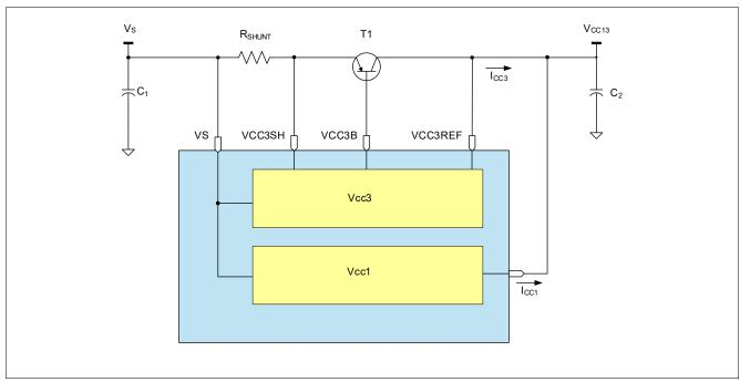
Figure 25 **VCC3 in Load Sharing Configuration**
