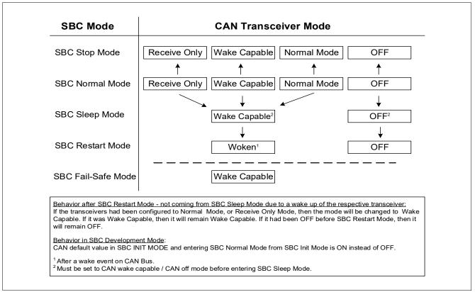
Figure 31 CAN Mode Control Diagram
