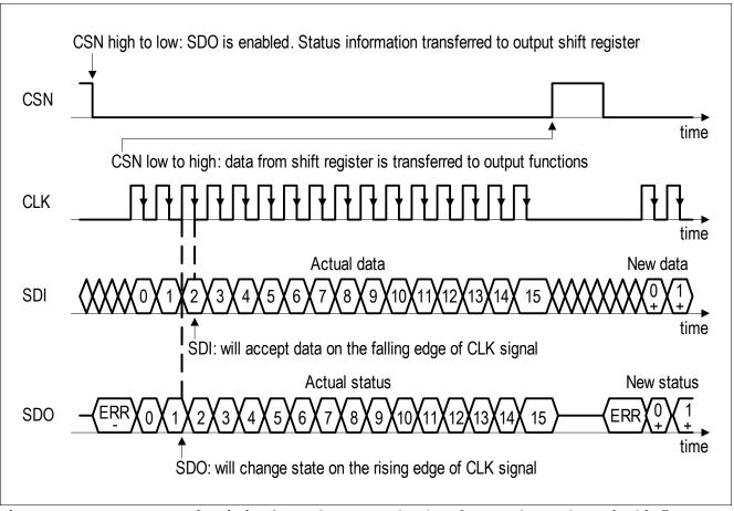
SPI Data Transfer Timing (note the reversed order of LSB and MSB shown in this figure Figure 53 compared to the register description)
