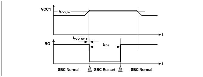
Figure 52 VCC1 Overvoltage Timing Diagram
