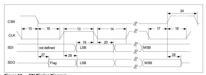
Figure 57 SPI Timing Diagram
