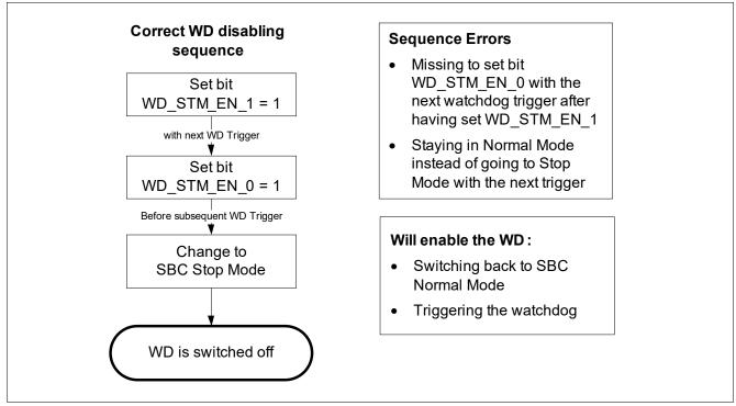
Figure 49 Watchdog disabling sequence in SBC Stop Mode
