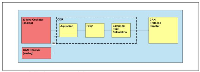
Figure 15 Clock and Data Recovery Block Diagram
