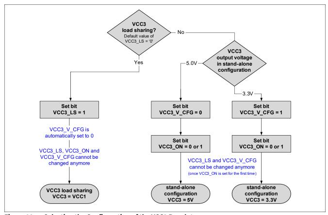
Figure 23 Selecting the Configuration of the VCC3 Regulator
