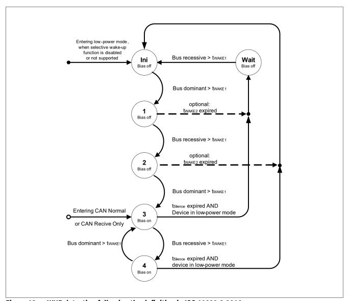
Figure 13 WUP detection following the definition in ISO 11898-2:2016
