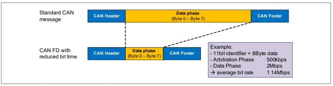
Figure 32 Bite Rate Increase with CAN FD vs. Standard CAN
