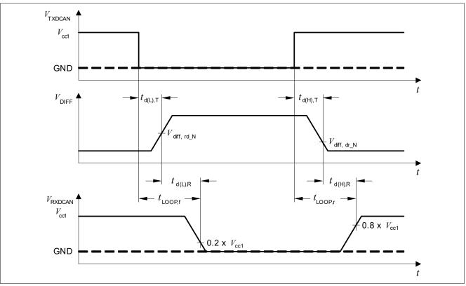
Figure 35 Timing Diagrams for Dynamic Characteristics
