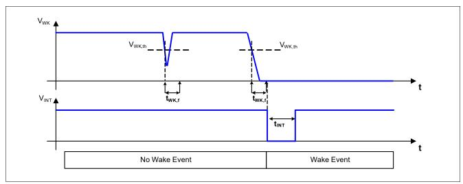
Figure 38 Wake-up Filter Timing for Static Sense
