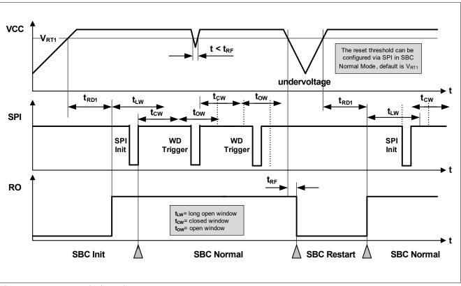
Figure 46 Reset Timing Diagram
