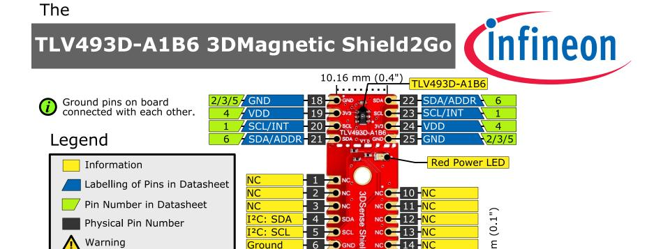
The maximum voltage on any pin is 3.5 V.
