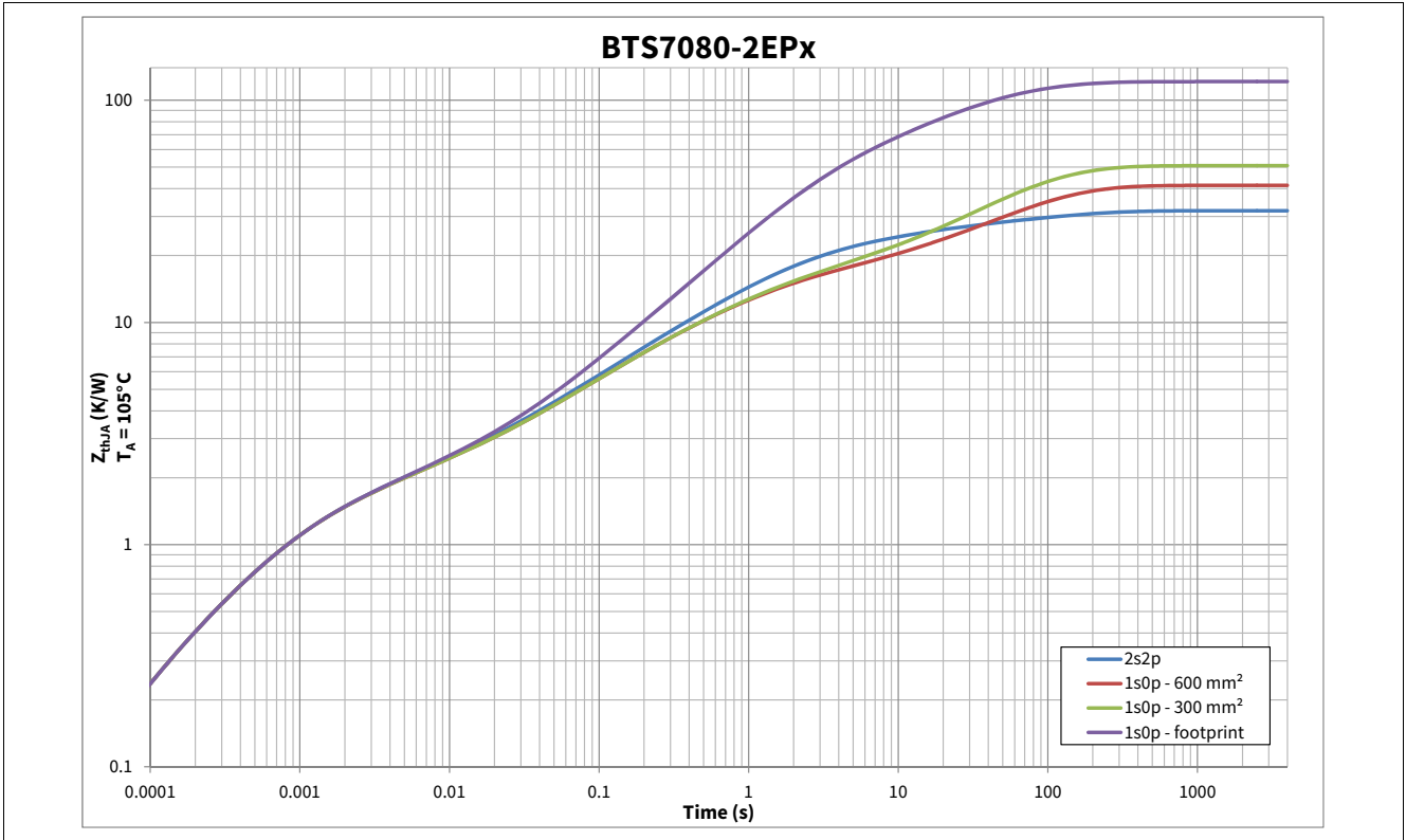
Figure 9 Typical Thermal Impedance. PCB setup according Chapter 4.4.1
