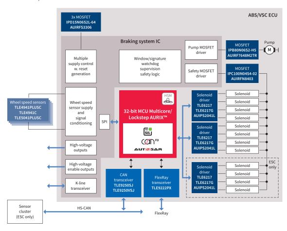
Thanks to its state-of-the-art safety features, the new TriCore™ AURIX™ family enables systems to achieve the highest ASIL-D safety level, which is already required in contemporary braking systems. The latest diverse lockstep technology with clock delay (diverse lockstep core) significantly reduces the software overhead and enables fast time-to-market. The scalability supports an optimized cost-performance fit for basic ABS systems up to highly integrated ESC systems.
