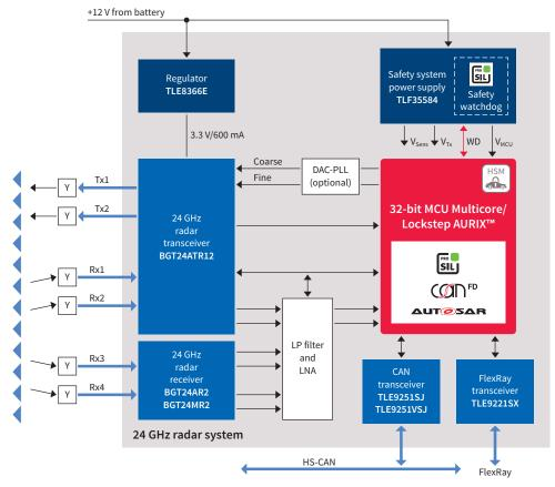
The new TriCore™ AURIX™ family will enhance classic safety features with dedicated features to meet the needs of 24 GHz radar systems. The combination of new features and increased SRAM, in conjunction with outstanding safety features, enables a high level of integration and reduction of complexity.
