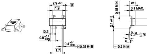
Note: Mold flash, protrusions or gate burrs of 0,2 mm max. per side are not included
