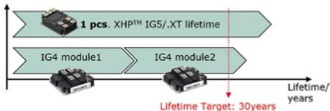
Figure 7: Comparison of lifetime for XHP™ 2 against two IHM modules
