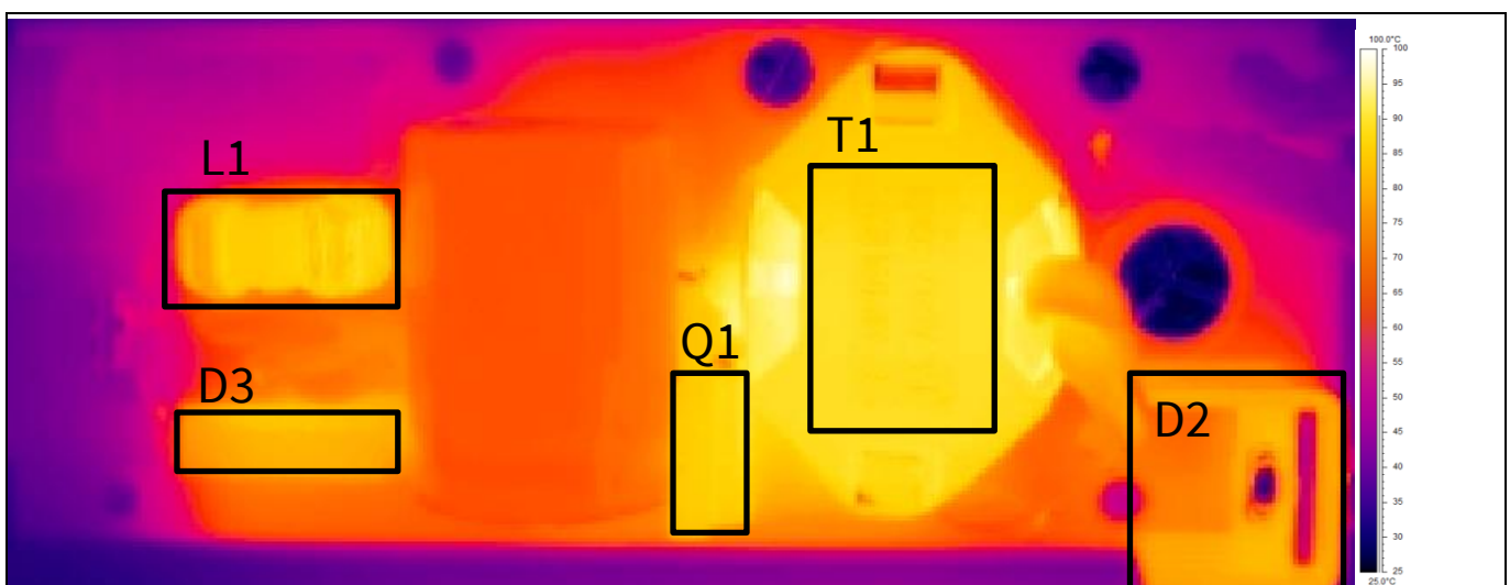
Figure 12 100 V AC input, full load, top side. The line filter and bridge rectifier are hottest at this point due to higher AC input currents.
