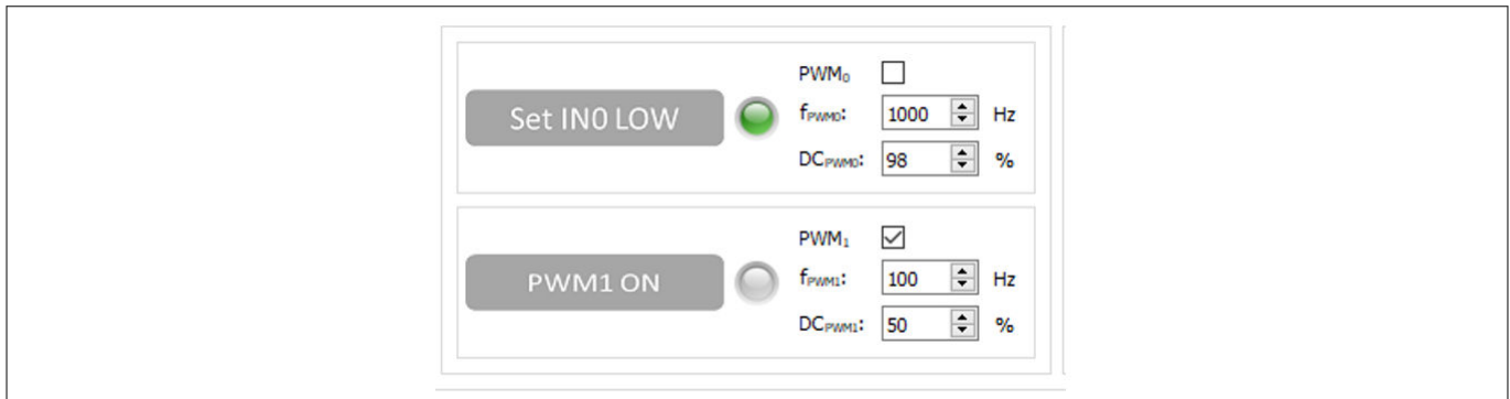
Figure 28 PROFET™ +2 12V functional view: – IN0 as logic input, IN1 as PWM input
