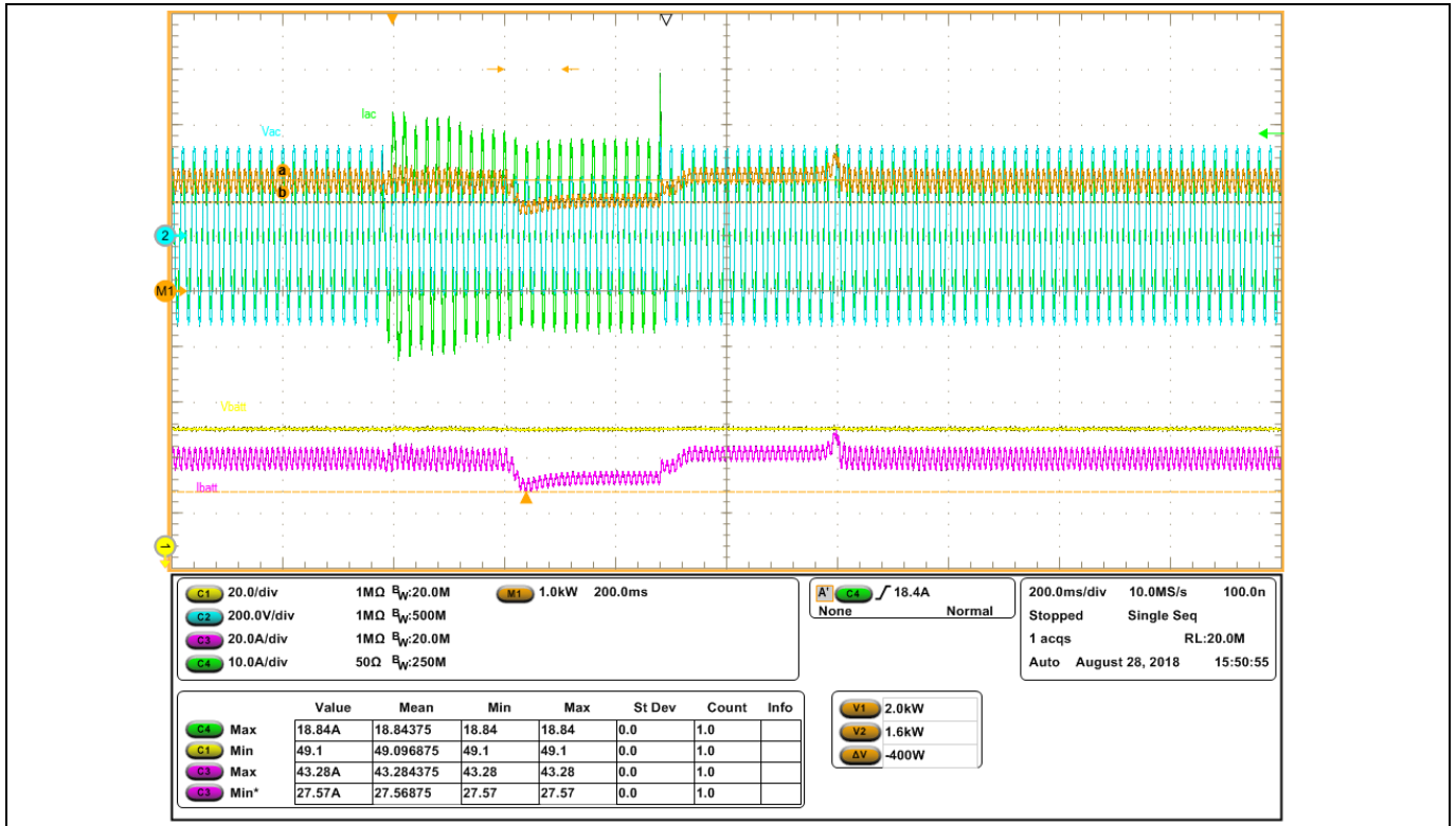
Figure 32 500 ms voltage dip with a voltage decrease down to 130 V AC
