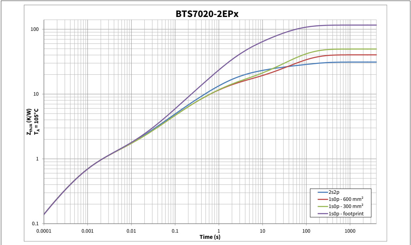
Figure 9 Typical Thermal Impedance. PCB setup according Chapter 4.4.1
