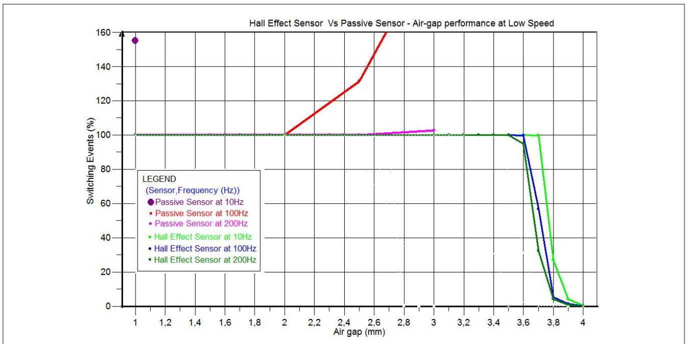
Figure 10 Air-gap performance at low rotational speed: Y-axis indicates the amount of recognized pulses for one revolution
