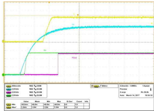
Start up at 16 A Load Ch1:V out , Ch2:PV in , Ch3:P Good , Ch4:V cc
