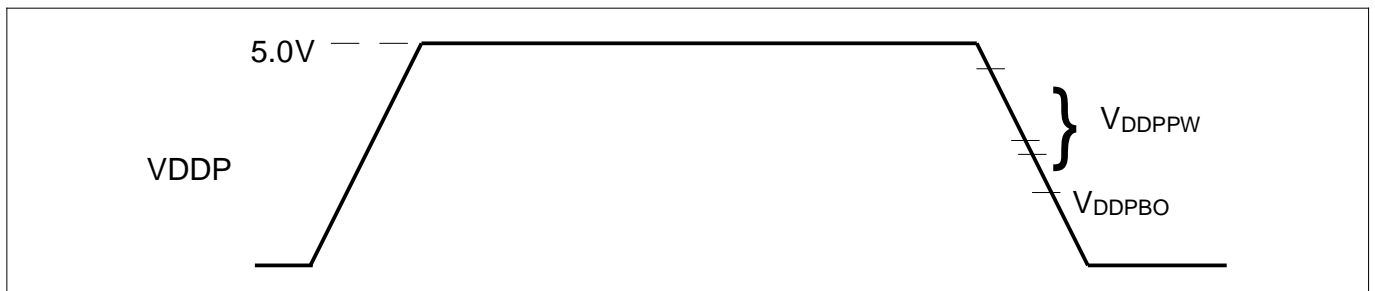
Figure 14 Supply Threshold Parameters
