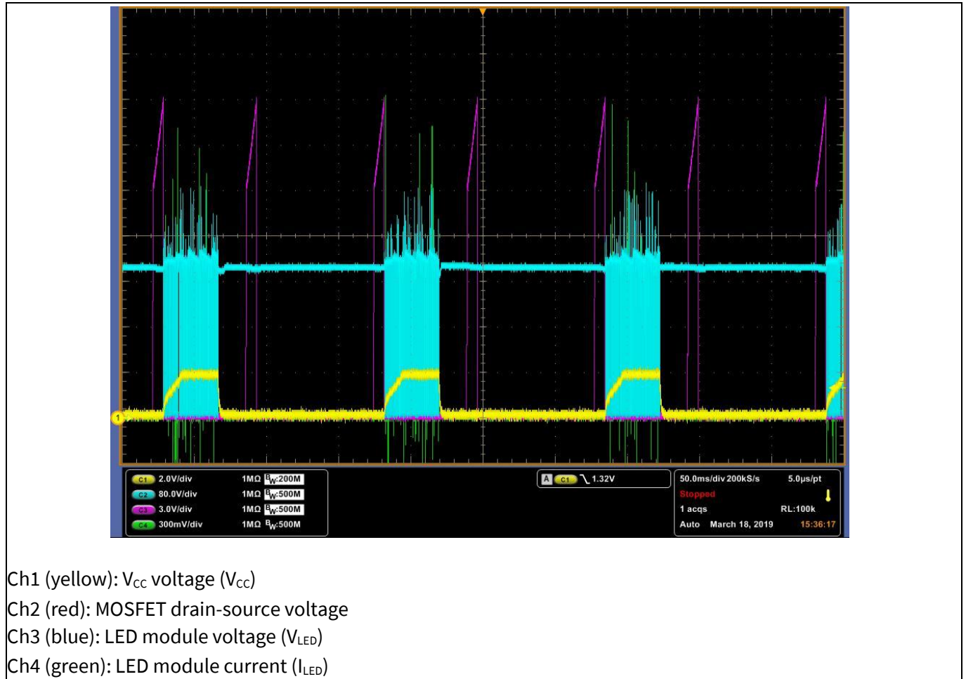
Figure 18 Short-circuit waveform during run mode at single-phase 230 V AC_{in}
