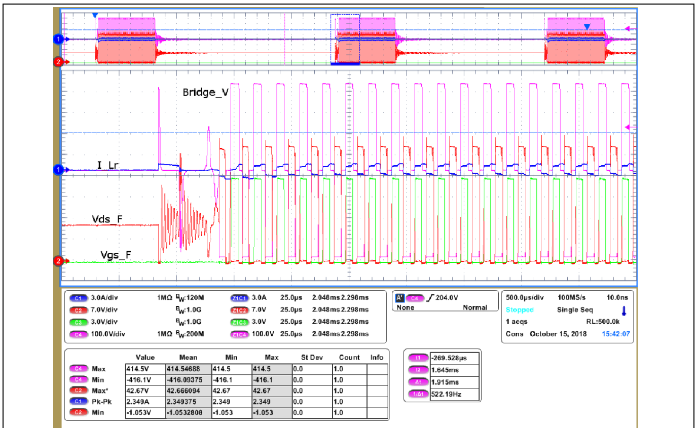
Figure 23 Burst operation with pre-charge of bootstrapping capacitors
