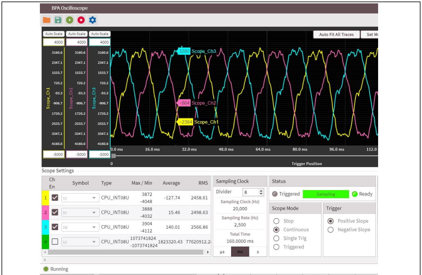
Figure 5 V/f open loop IU, IV, IW current waveform captured by the GUI's oscilloscope
