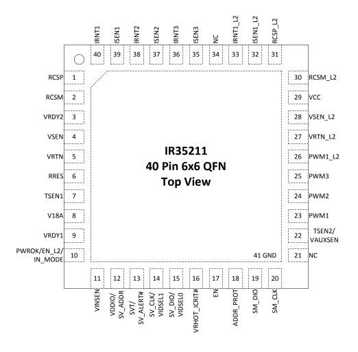
Figure 1: IR35211 Pin Diagram
