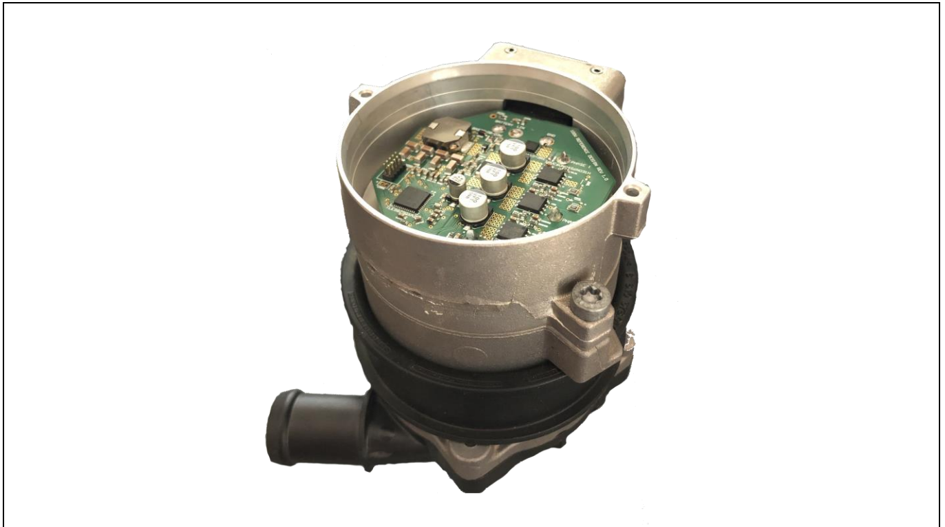
Figure 1 PCB in pump housing
