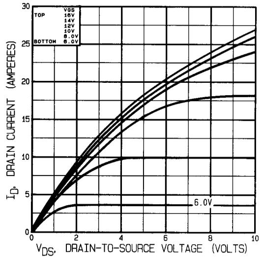
Fig 14. Typical Output Characteristics Post-Irradiation 100K Rads (Si)
