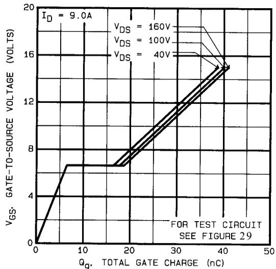
Fig 22. Typical Gate Charge Vs. Gate-to-Source Voltage
