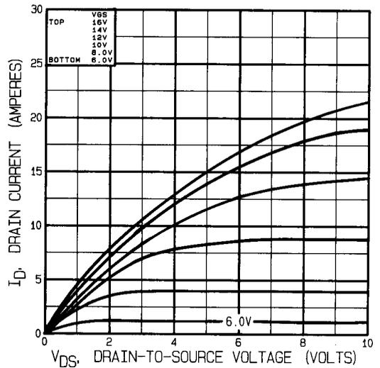
Fig 16. Typical Output Characteristics Post-Irradiation 1 Mega Rads (Si)
