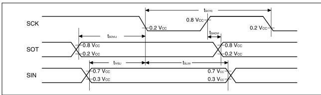
Sampling is executed at the falling edge of the sampling clock\*1, and serial clock delay is enabled\*2. (ESCR register : SCES bit = 1, ECCR register : SCDE bit = 1)
