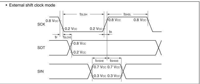
Sampling is executed at the falling edge of the sampling clock<sup>\*1</sup>, and serial clock delay is disabled<sup>\*2</sup>. (ESCR register : SCES bit = 1, ECCR register : SCDE bit = 0)
