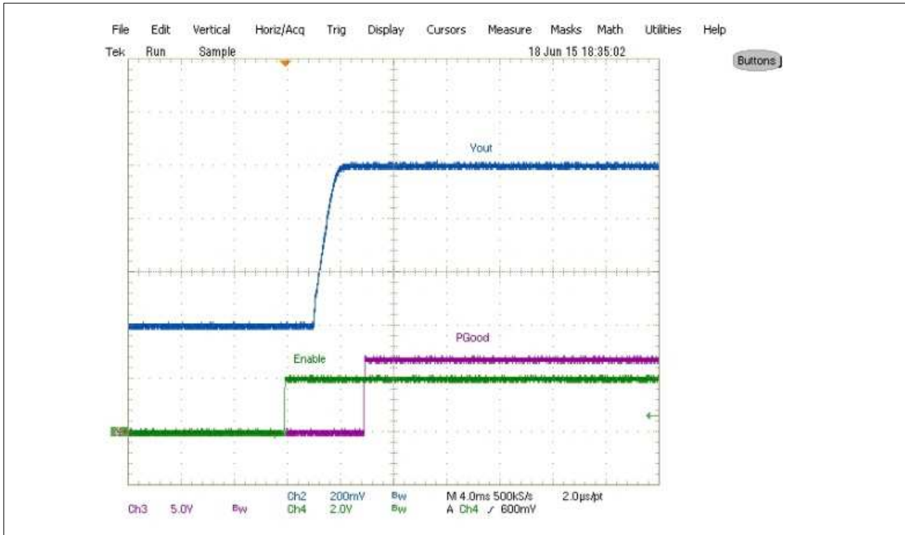
Figure 7-9 Start up with pre bias, 0A Load (Ch 2 :Vout, Ch 3 : PGood, Ch 4 :Enable)
