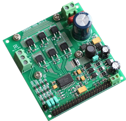
The 76 x 83mm board has two layers with 1oz (~35µm) copper each.
