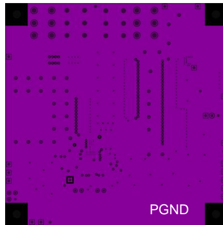
Figure 51c: IRDC3846 Demo board Layout Considerations – Mid Layer 1
