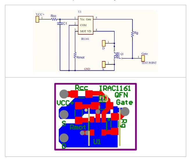
The daughter card shown above is designed to allow easy retrofit in existing systems with minimal system changes. The component values are recommended but user has freedom to change them per application requirement.
