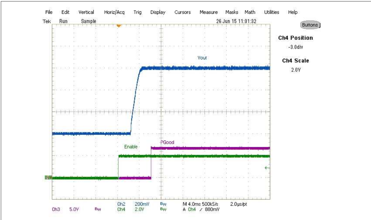
Figure 7-8 Start up with pre bias, 0A Load (Ch 2 :Vout, Ch 3 : PGood, Ch 4 :Enable)
