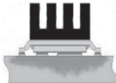
③ Mounted to a PCB with small clip heatsink (still air)
