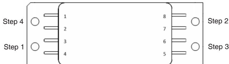
Figure 2. Top view of the HTB Converter with tightening sequence
