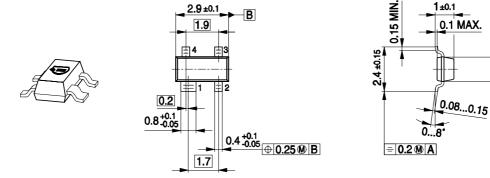
Note: Mold flash, protrusions or gate burrs of 0,2 mm max. per side are not included
