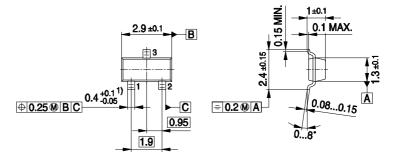
1) Lead width can be 0.6 max. in dambar area
