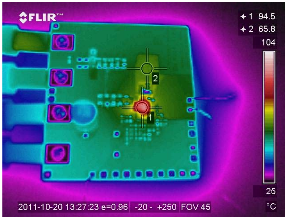
Figure 46: Thermal Image of the Board at 16A Load, Test Point 1 is IR3895, Test Point 2 is inductor
