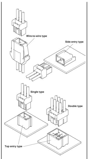
This PSI connector is designed for wire-toboard and wire-to-wire 4.0 mm pitch connector. Low insertion force type contact is adopted and it provides excellent operability. This connector has the secure locking device that has the mechanism for preventing the inverse insertion. By adopting key shape and multi colors of housing, prevention function of mis-mating is considered.
