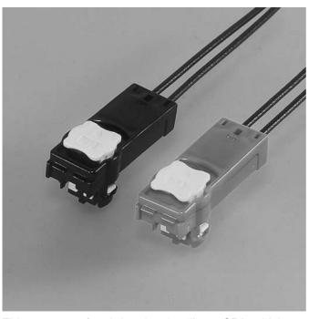
This connector for air-bag has intelligent CPA, which allows locking the connector, incomplete mating detection and release of short-circuit at the same time.
