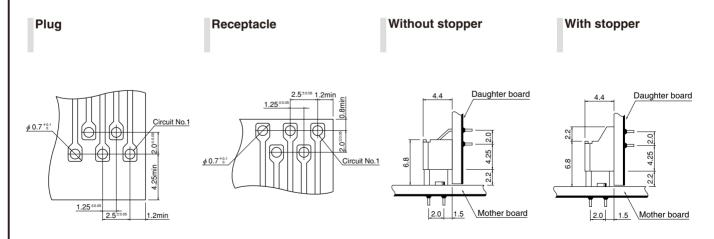
Note: 1. Tolerances are non-cumulative: ±0.05mm for all centers. 2. Hole dimensions differ according to the kind of PC board and piercing method. The dimensions above should serve as a guideline. Contact JST for details.
