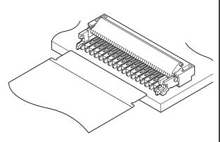
0.2 mm pitch FVXS connector for FPC has been developed for small portable equipment for which low profile and miniaturization are required. Positioning of FPC is easily conducted by inserting FPC into connector until its shoulder touches to the transverse U-shape groove.
