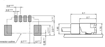
Note: 1. The above figure is the figure viewed from the connector mounting side.
