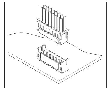
This is a 2.0mm pitch, crimp style, doublerow, wire-to-board connector. It is designed to meet the demand for highdensity and low-profile connection.
